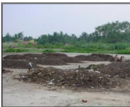
Raw MSW dumped in the platform for preparing the waste for Vermicompost pits at Bhadreswar Municipality
