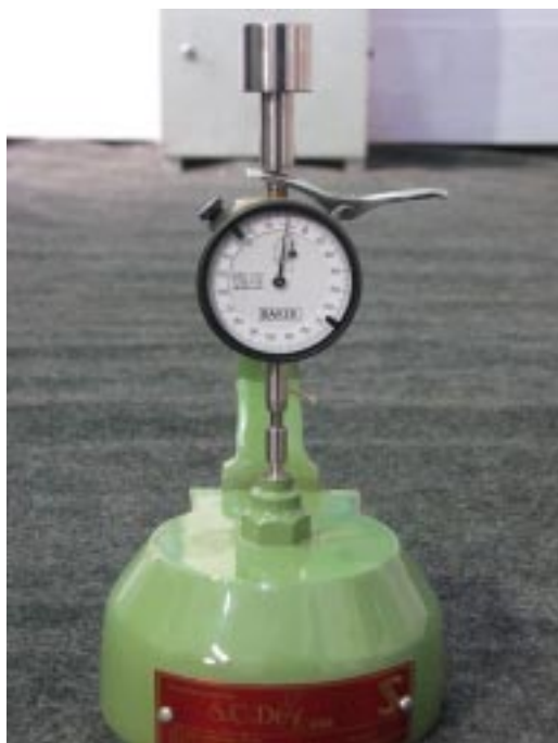
Gauge Meter is used for measuring the thickness of plastic carry bags
