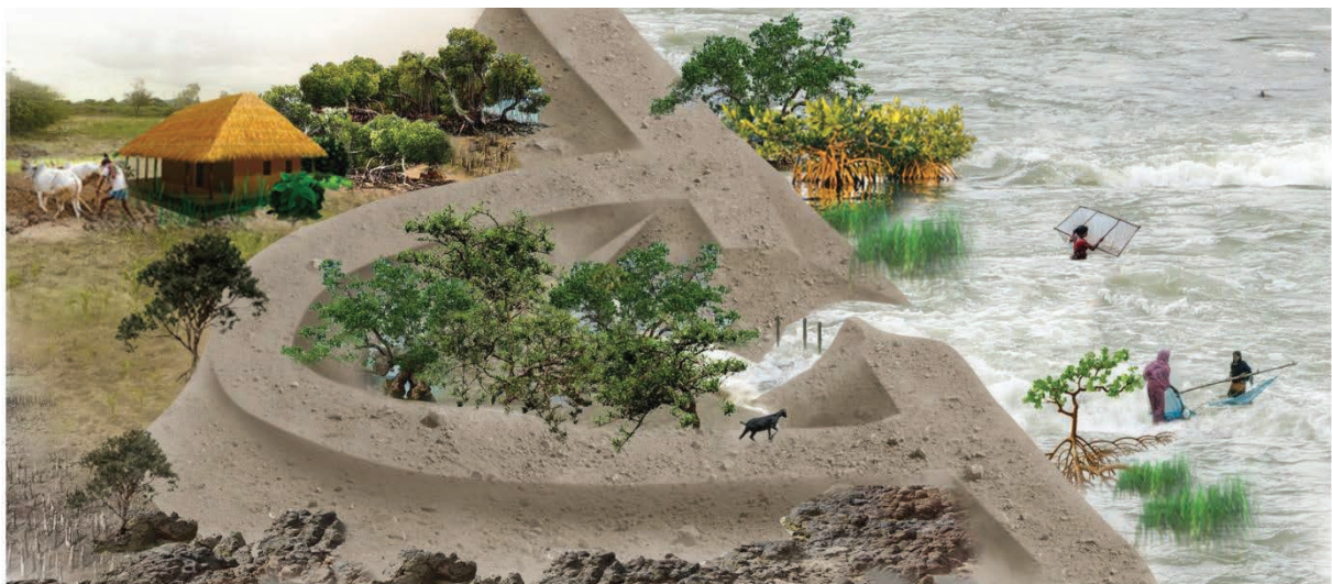
Fig. 20 The proposed retired embankment as second line of defence.
