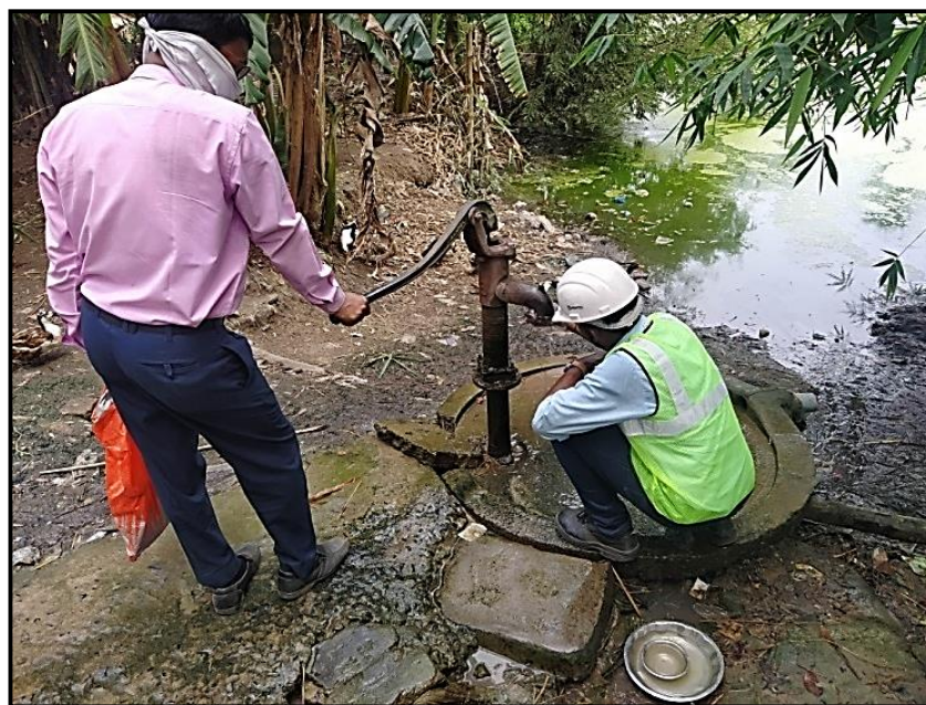
Figure 3-16: Ground Water Sampling
