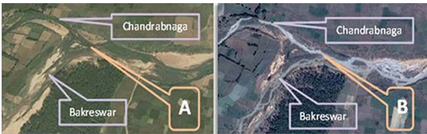
Figure 24.31 :Confluence of rivers Chandrabnaga and Bakreswar before (A) and after (B) the incident of ash pond overflow.
