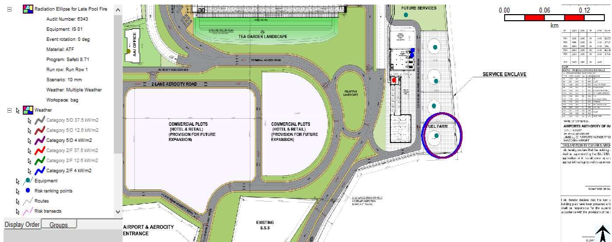
Figure 7.15: Pool Fire (10 mm) Consequence Contour for Blowout Scenario (IS 01)
